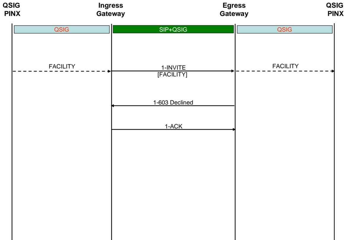
Figure 4 — QSIG call independent connectionless signalling
