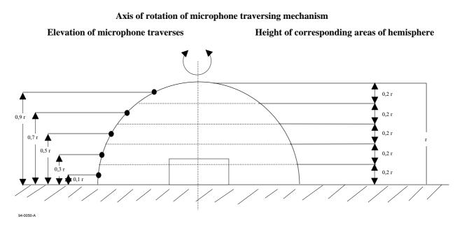
In this arrangement either the microphones or the equipment may be rotated.
