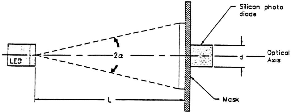
Figure A.1 - Optical Arrangement
