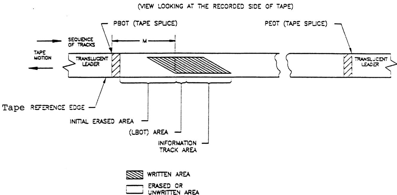
**Figure 28 Physical Tape Layout**
