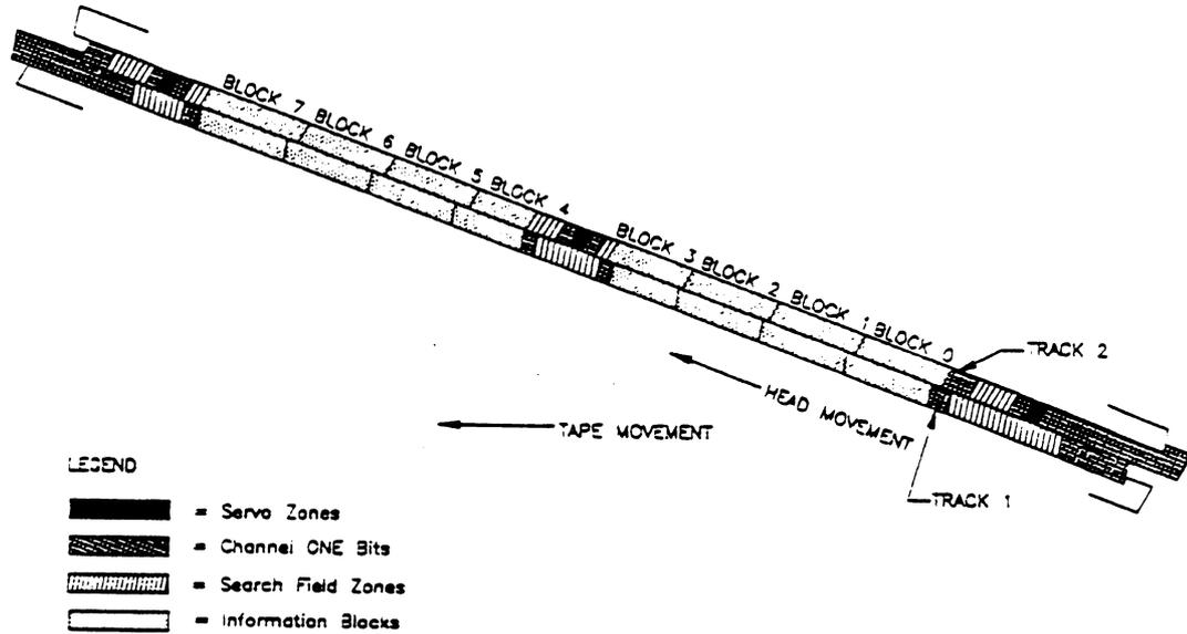
Figure 26 - T1 and T2 Track Layouts
