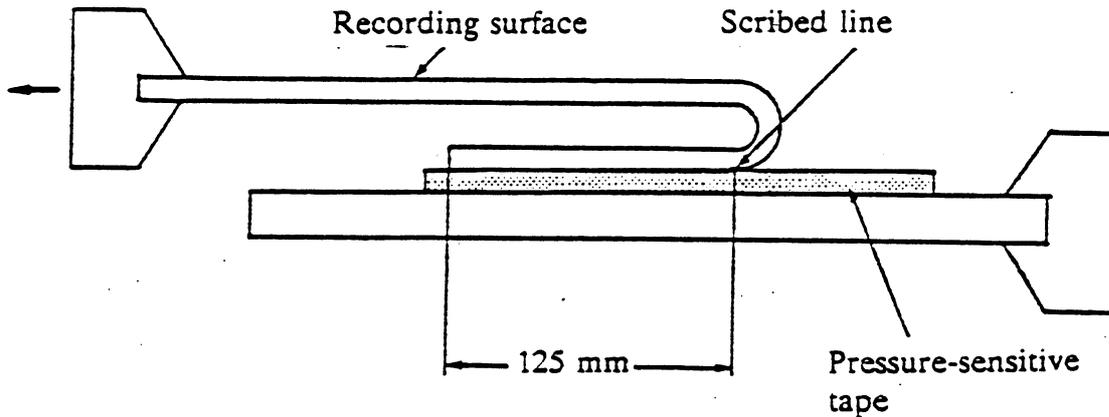
Figure 20 - Setup for Measuring Coating Adhesion
