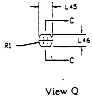
Figure 6 - Details of Datum and Recognition Holes
