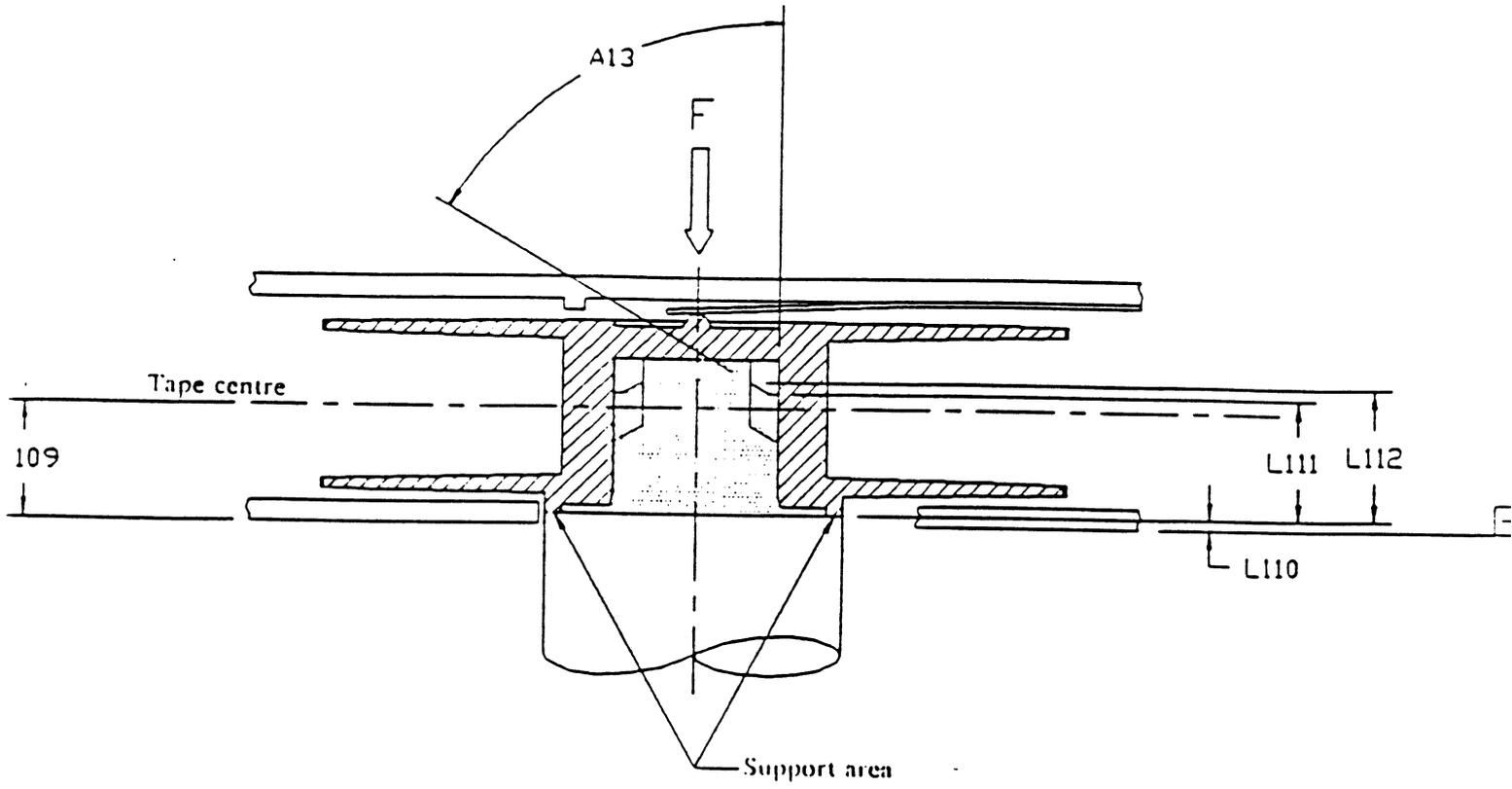
Figure 18 - Interface with Drive Spindle
