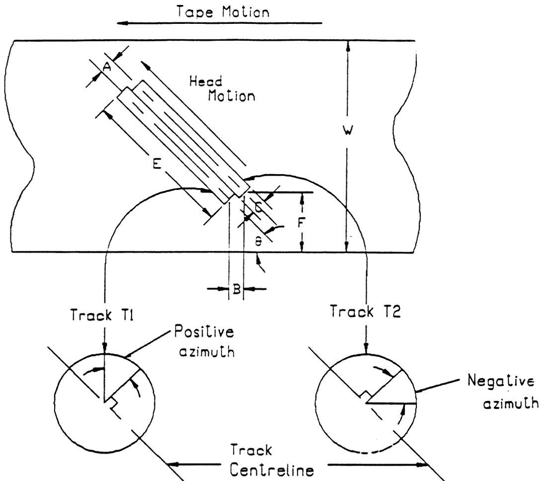
Figure 23 - Track Layout and Track Location
