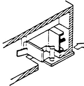
**Figure 12 - Direction of Force Needed to Unlock the Reel Lock**
