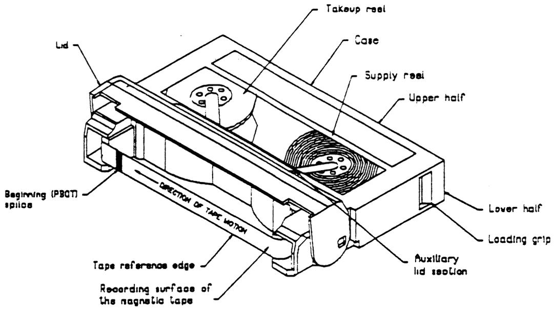
Figure 1 - Tape Cartridge Assembly Top View (Lid Open)
