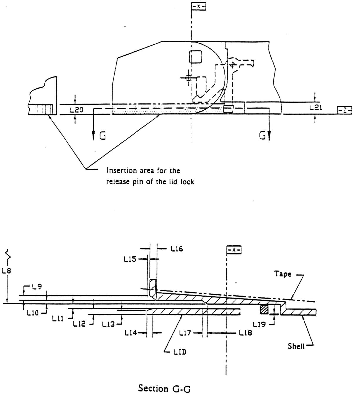
Figure 9 - Lid Release Insertion Channel
