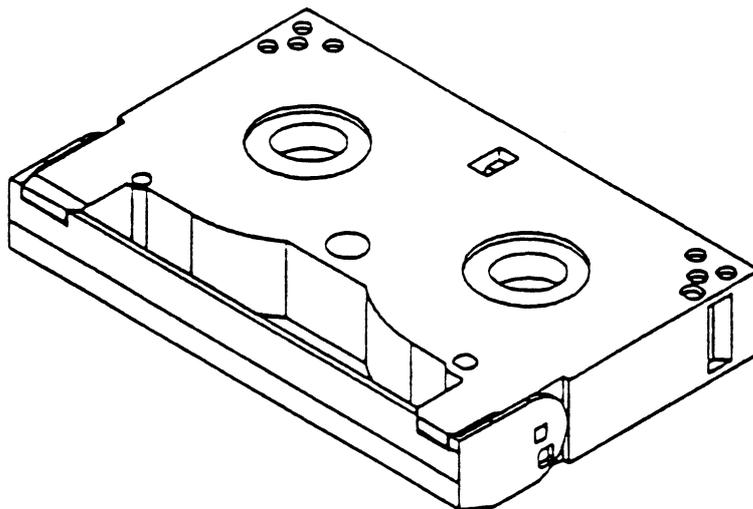
Figure 2 - Tape Cartridge Assembly Bottom View (Lid Closed)
