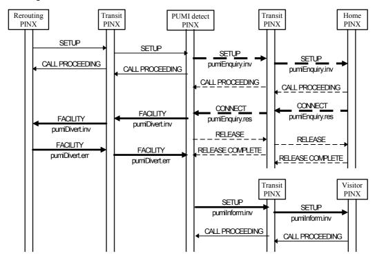
Figure C.2 - Example of forward switching by the PUMI-detect PINX
