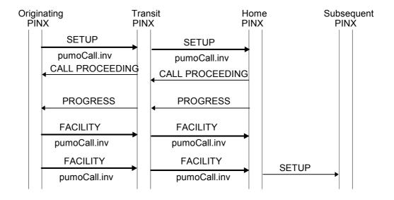
Figure C.6 - Successful invocation of ANF-PUMO with overlap operation
