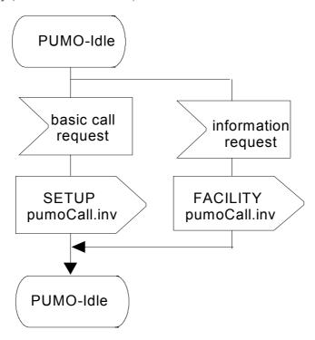
Figure D.5 - Originating PINX behaviour
