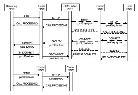
Figure C.1 - Example of normal operation of ANF-PUMI
