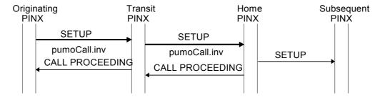
Figure C.7 - Successful invocation of ANF-PUMO with en-bloc operation
