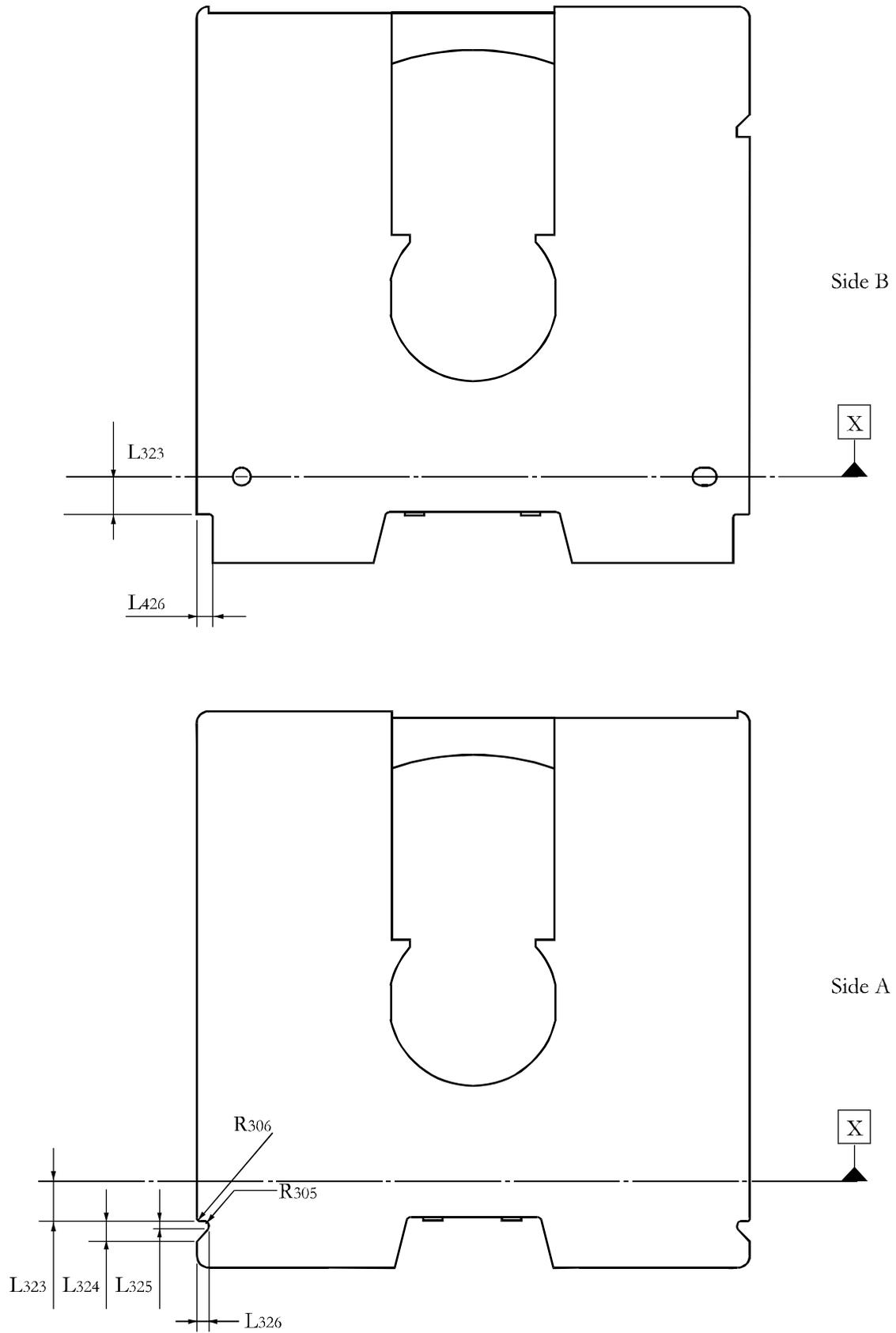
Figure 49 – Mis-release protection function of body of the case
