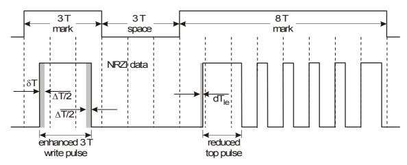
Figure F.2 - Example of a Multiple-pulse
