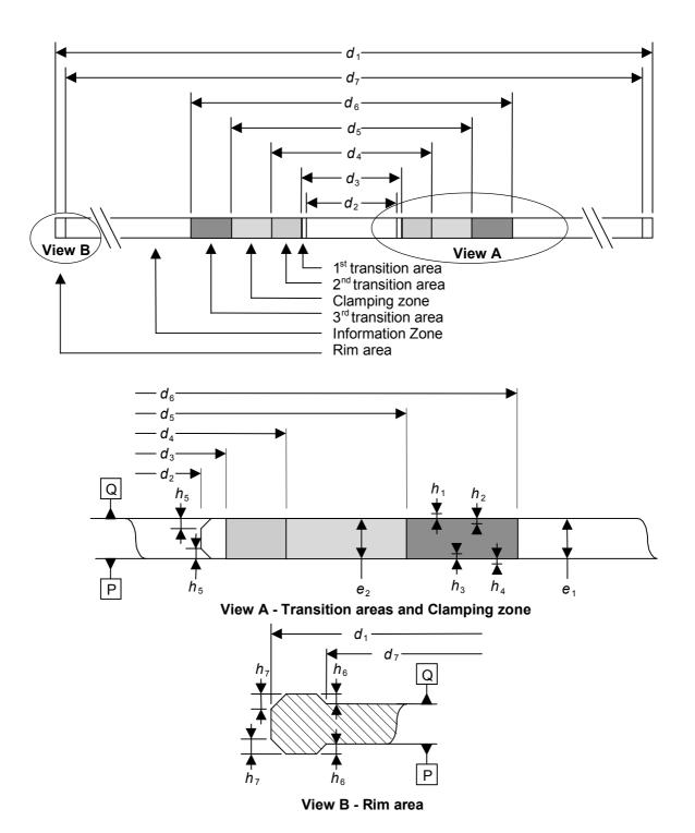
Figure 7 - Physical disk dimensions
