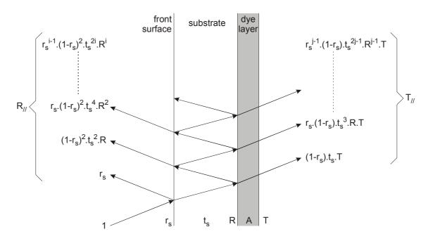
Figure J.2 – Definitions of reflectivity, transmission and absorption
