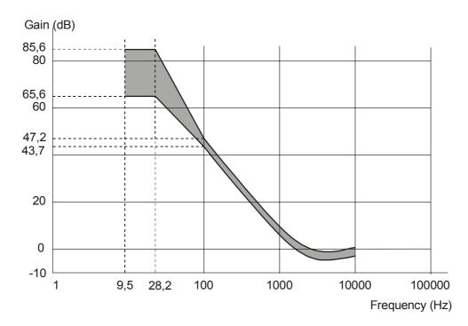
Figure 5 - Reference servo for radial tracking
