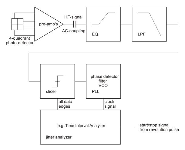
Figure D.1 - General diagram for jitter measurement
