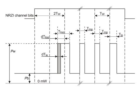
Figure F.1 - Write pulse waveform
