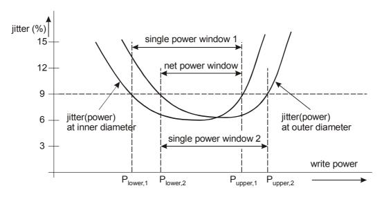
Figure 31 - Example of the write power windows
