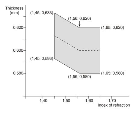
Figure 8 - Thickness of the substrate
