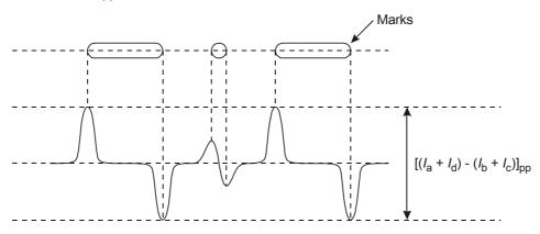
Figure 35 - Tangential push-pull signal
