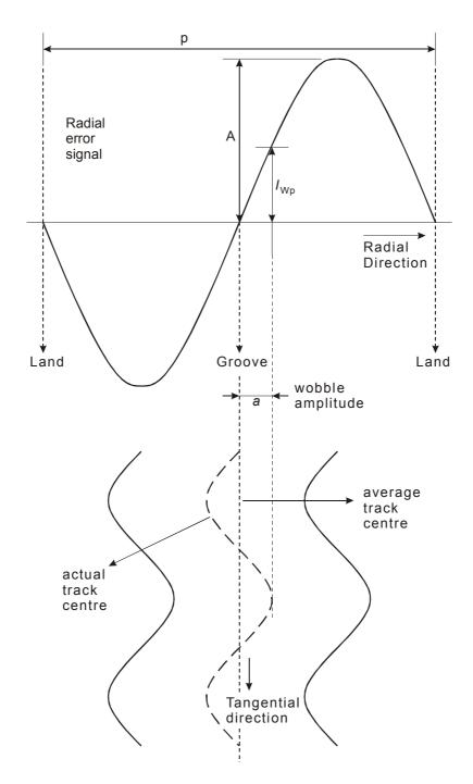
Figure M.1 - Wobble amplitude of the groove
