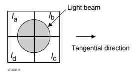
Figure 33 - Quadrant photo detector
