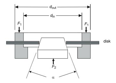
Figure 3 - Clamping and chucking conditions
