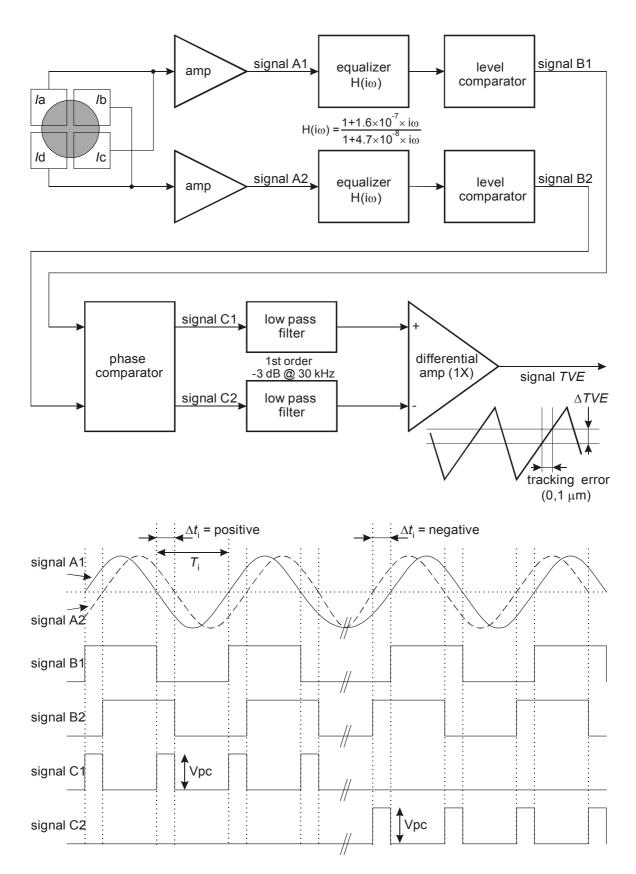
Figure E.1 - Circuit for tracking error measurements
