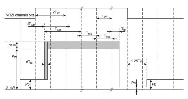
Figure F.3 – General blocked waveform
