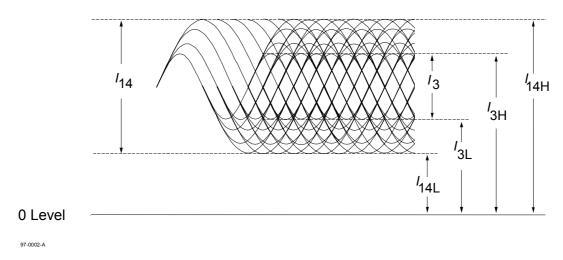
Figure 32 - Signals from spaces and marks in Read channel 1
