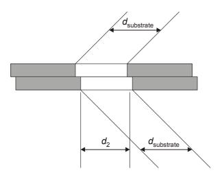
Figure 6 - Hole diameters for an assembled disk
