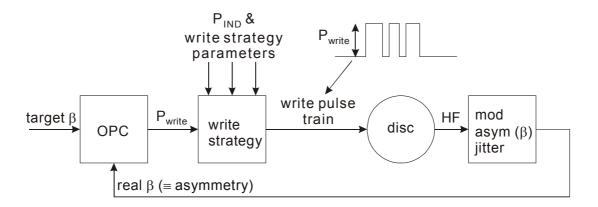
Figure H.1 - Schematical diagram of OPC procedure
