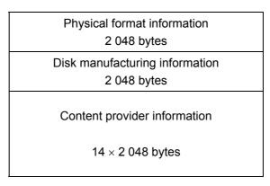
Figure 26 - Structure of a Control Data Block
