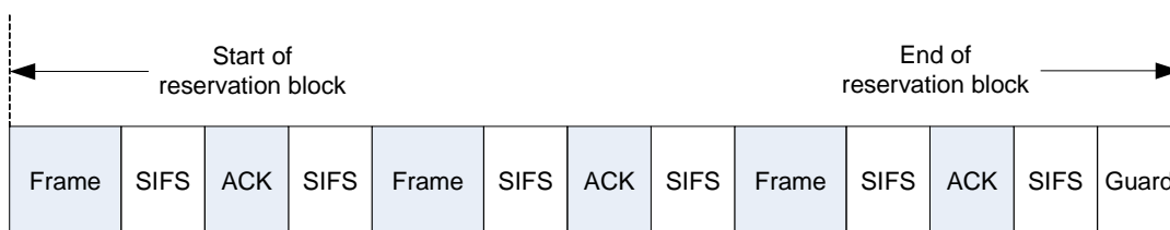
Figure 168 - SIFS and guard time in a DRP reservation block - Imm-ACK
