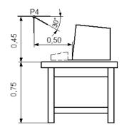
b) Seated operator for table-top equipment (case 2: without keyboard)
