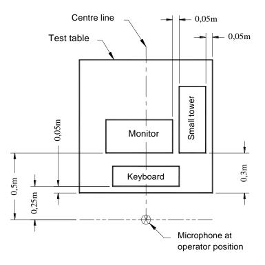
Figure C.4b — Installation for a small tower table-top system
