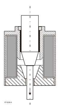
Figure A.3 — Solenoid cross section
