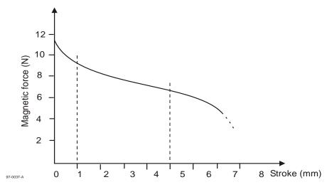
Figure A.2 — Solenoid characteristics for a plunger stroke of 4 mm
