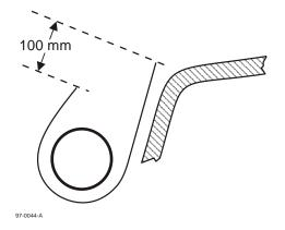
Figure C.1 — Insertion of single sheet of paper
