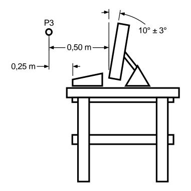
Figure C.4d — Screen angle for all-in-one system
