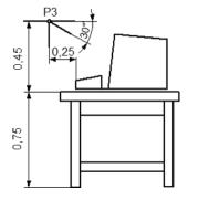
a) Seated operator for table-top equipment (case 1: with keyboard)
