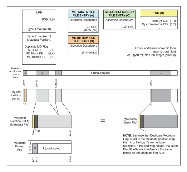
**NOTE:** the LBN values used in the diagram above are for illustrative purposes only and <u>are not</u> fixed. The partition references used <u>are fixed</u> as a consequence of the Metadata Partition implementation.
