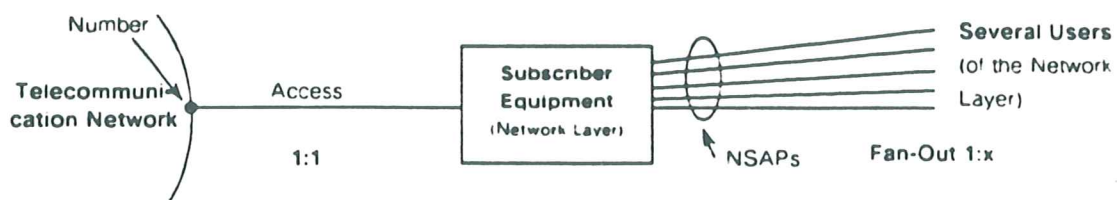
Figure 34 - NSAP Addressing Principle in OSI Endsystems
